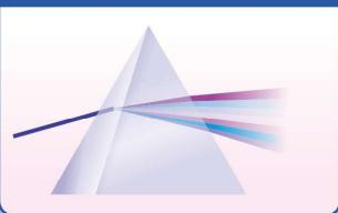
When light passes through prism it breaks into seven colors. These colors are present in light but only visible when prism is used.
